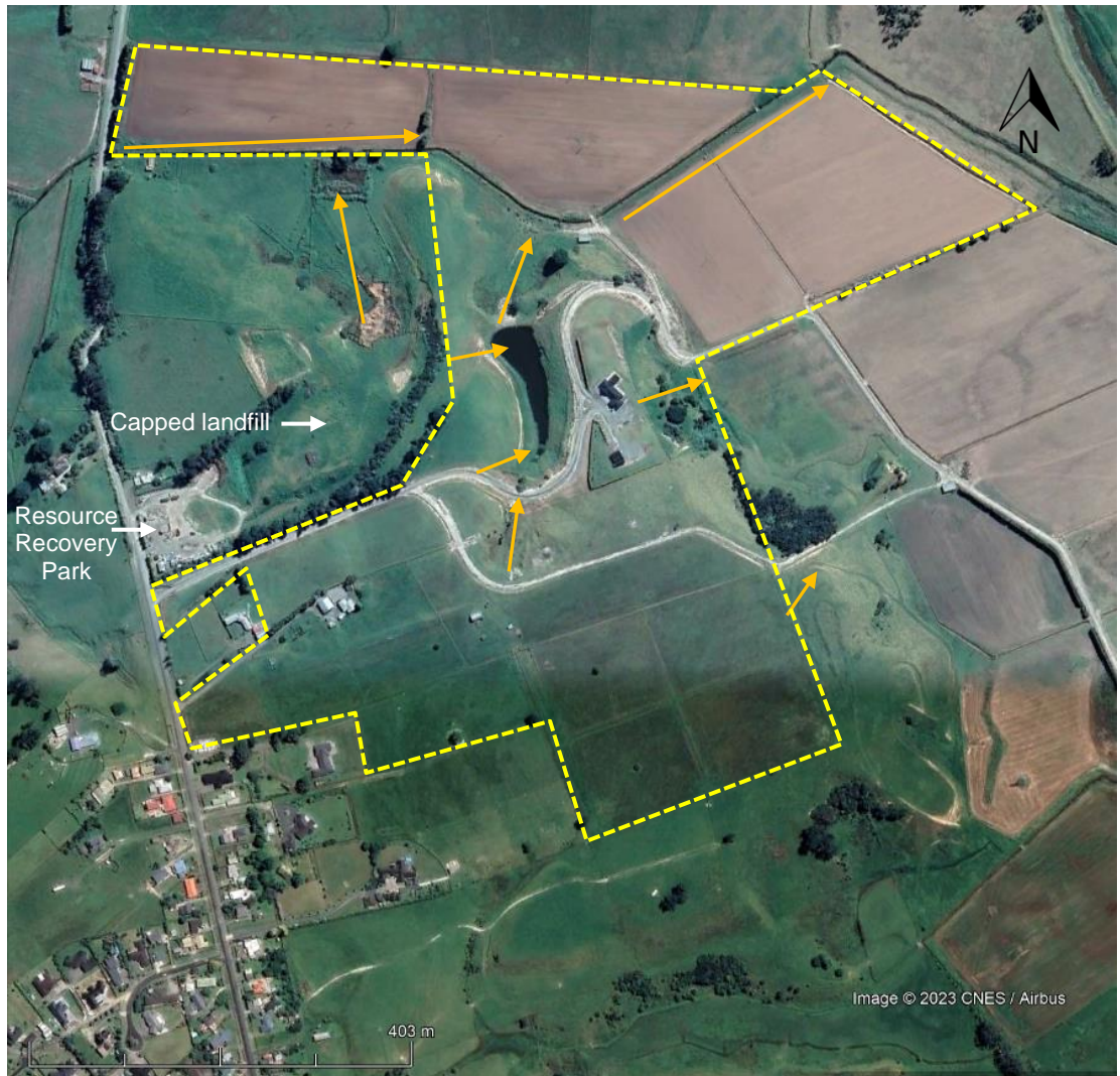
E 11 Aerial view taken 2022 showing indicative drainage patterns and contemporary land use (Source Google Earth)
